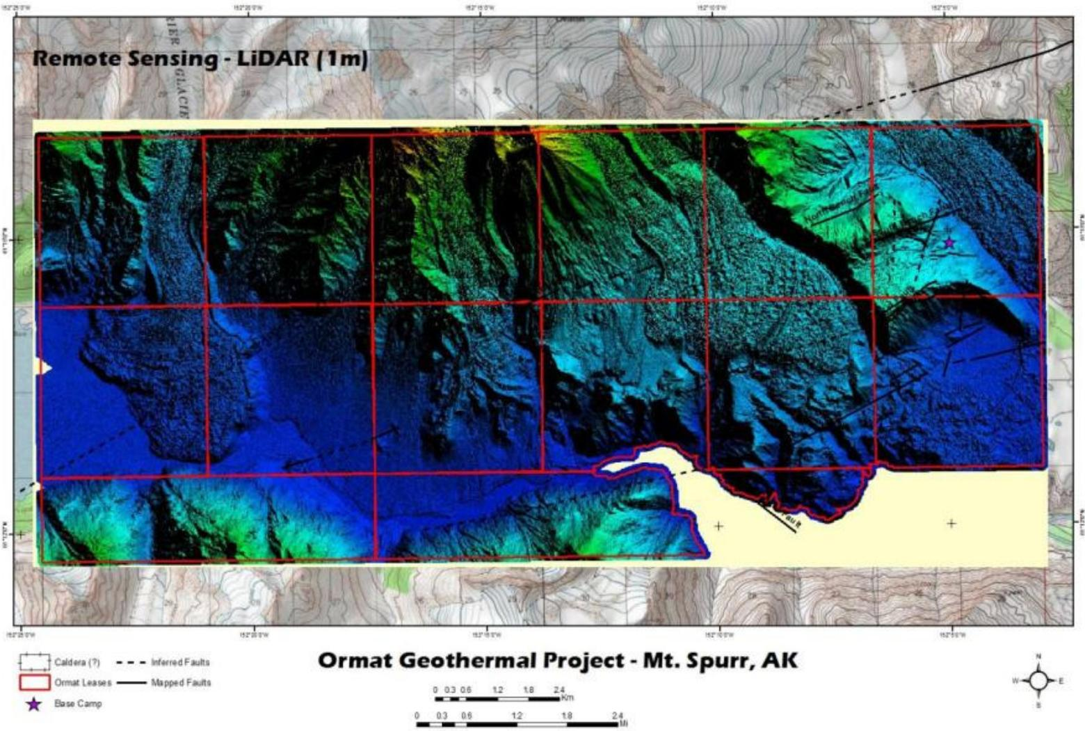
Figure 7: LiDAR data acquired over the Mt. Spurr geothermal leases at a binned 1m resolution. Cooler colors are lower elevation while warmer colors are higher elevations.
