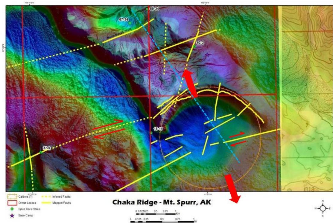
Figure 10: RTP magnetics overlaid on top of LiDAR data which is in turn overlaid on topo quads. Solid yellow fault/fracture segments are a combination of field-mapped faults and LiDAR-based mapping. Large red arrows highlight conjectured extension direction. Dashed blue line refers to line of section shown in Figure 11
