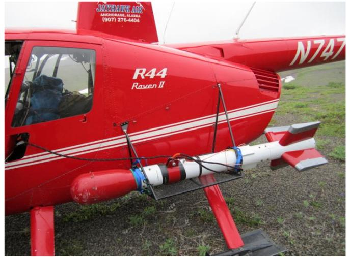
Photo 8: Heli-magnetic survey helicopter
