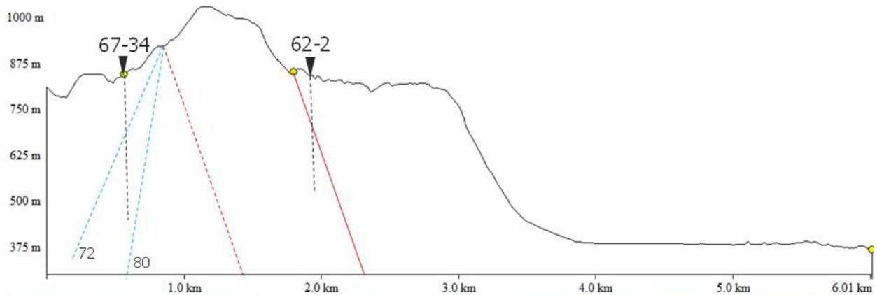
Figure 11: Cross-section showing location of core-holes and the intersected fault (solid line), originally projected faults (dashed blue lines) and currently projected fault (dashed purple line)
