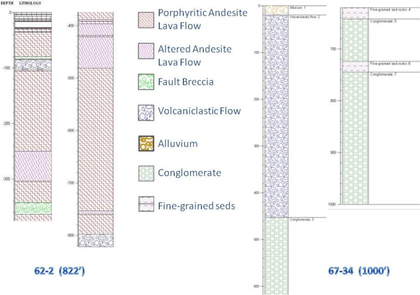
Figure 8: Lithology logs for both core wells 62-2 and 67-34
