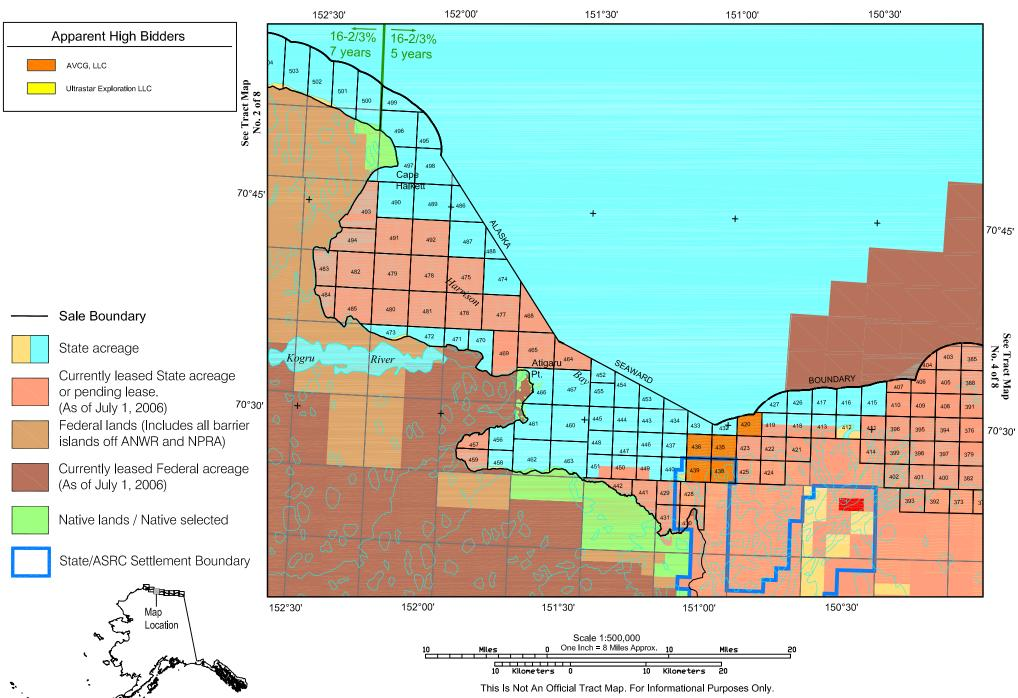
Albers Equal-Area Conic Projection, 1927 North American Datum, Clarke 1866 ellipsoid with a central meridian of 150° 45′, origin latitude of 50°, northern parallel of 65°, and southern parallel of 55°.
