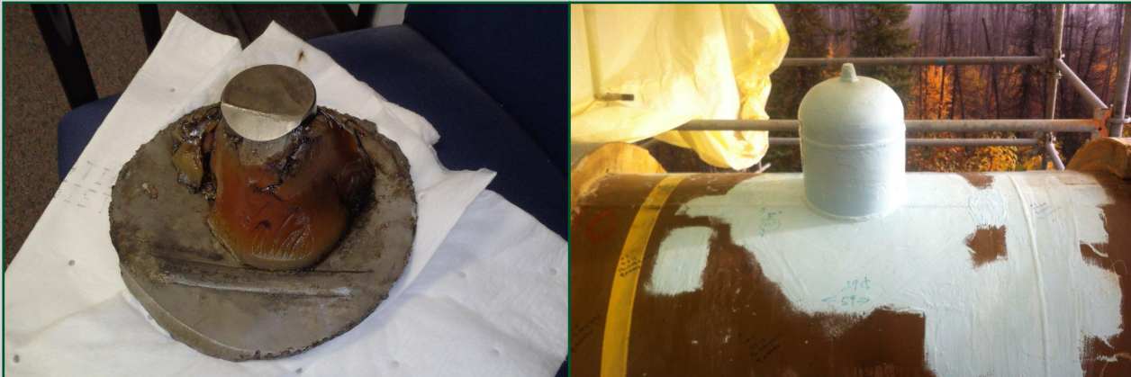
Left: Ten-inch diameter wall section with two-inch T-O-R, cap and epoxy (photo courtesy of APSC) Right: Dome-like encapsulation structure
