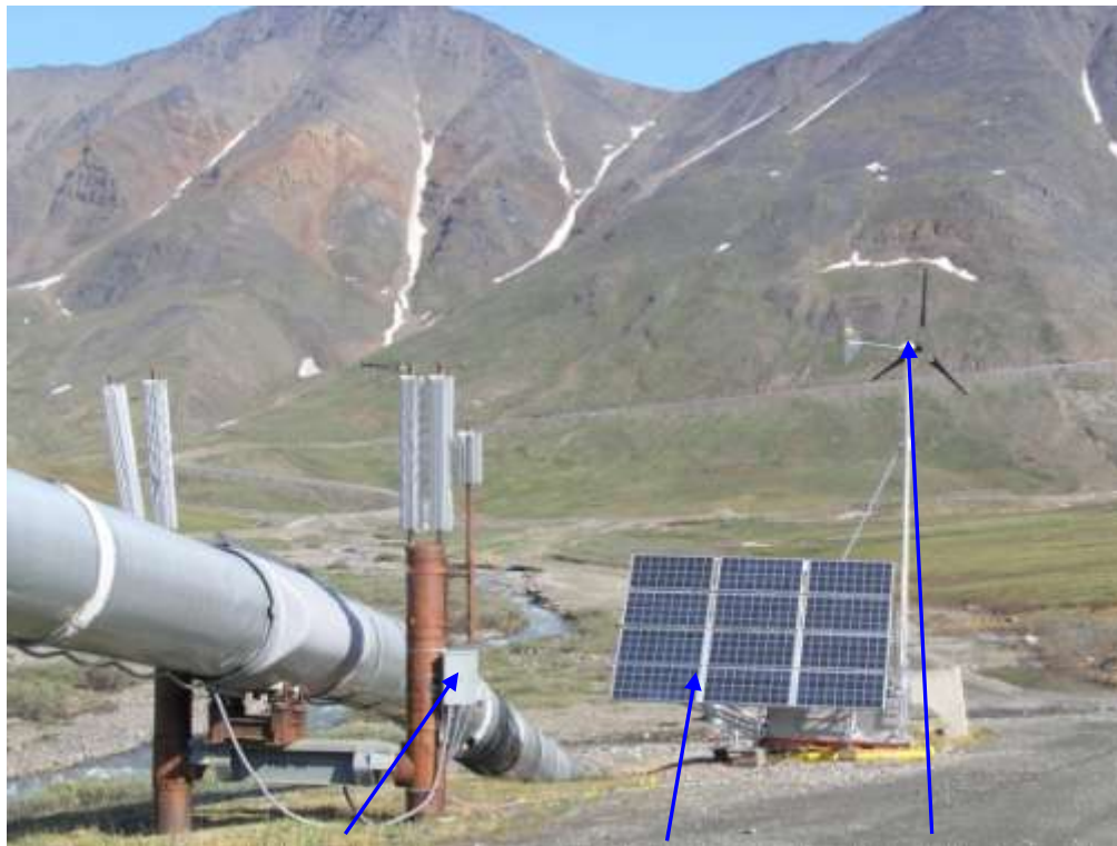
Figure 14: Data Logger Instrumentation , Solar Panel , and Wind Generator at Atigun Pass 9
