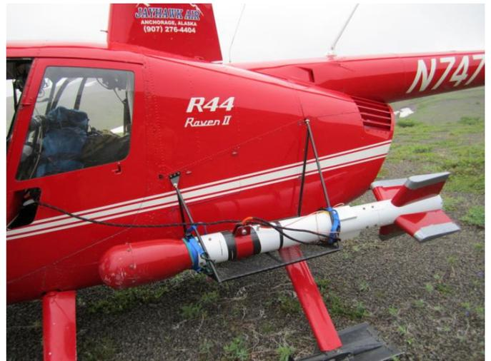
Photo 8: Heli-magnetic survey helicopter
